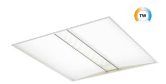
Illusion LED Tunable White is the next generation in dynamic lighting, making use of LED technology to give higher comfort and an even better environment for users – under the motto: "Bring the "daylight" indoors". Tunable White from 2700 Kelvin to 6500 Kelvin white light. Controlled by Dali Type 8.
